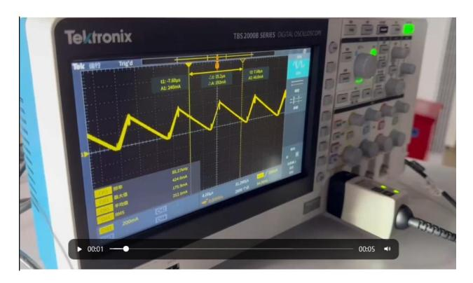
Regarding the evaluation, the waveform in the second image is correct. We tried to measure to check the waveform from 0Khz - 100Khz, the waveform from 20Khz onwards was distorted as shown in the attached image.
